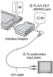
• If your TV has stereo input jacks, connect the audio plug (black) of the A/V cable to the left audio jack.
